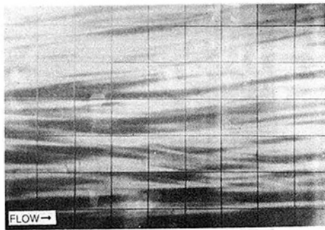
Fig. 8 Photograph of visualized streak pattern beneath turbulent boundary layer in recovery region
